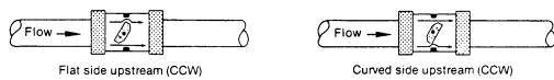
Figure 1. Valve positions with uniform inlet flow and counterclockwise (CCW) disc rotation on closure.
